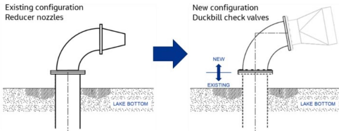
Figure 10.3 Existing and New Diffuser Port Configuration
