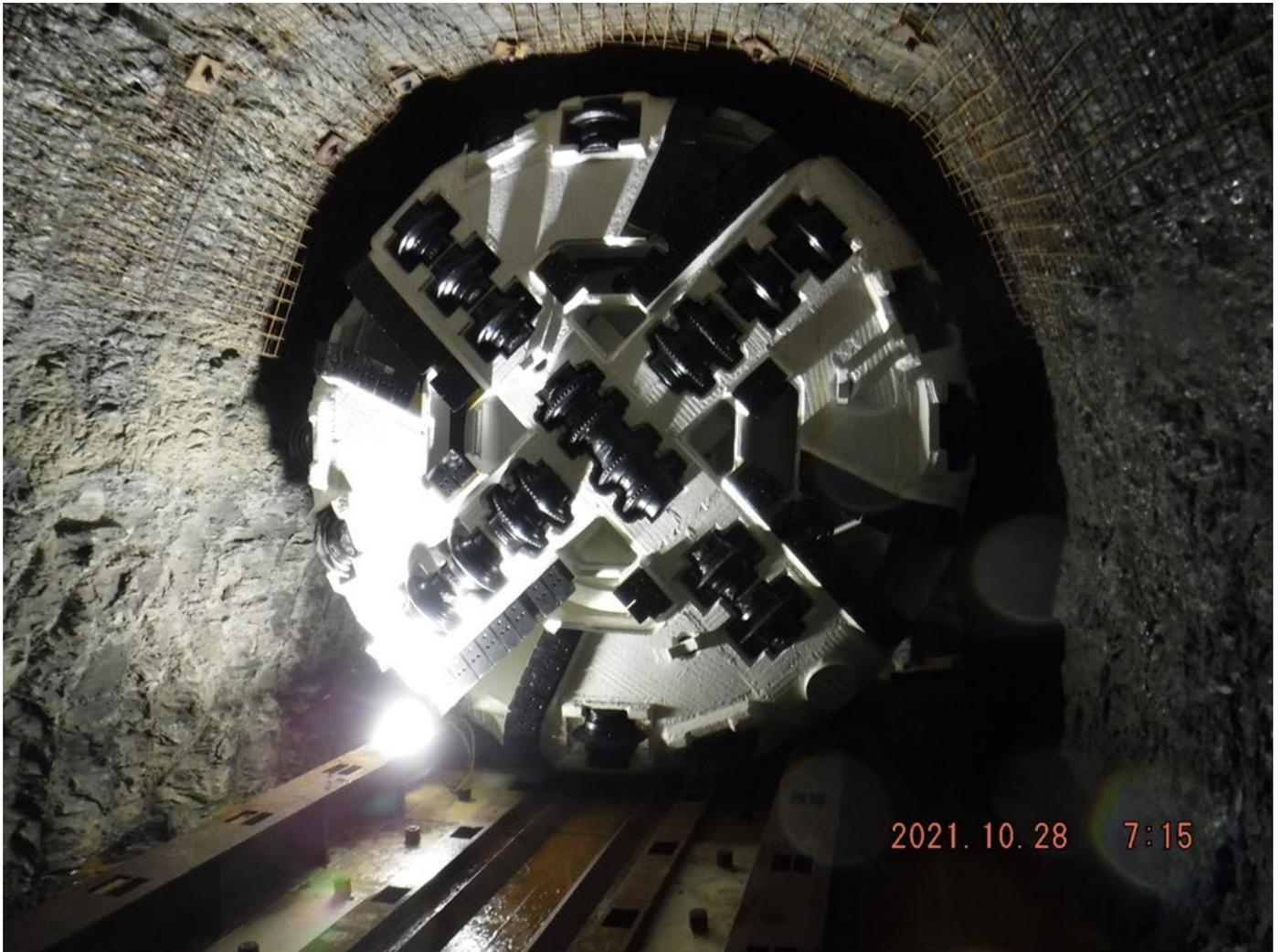
Figure 10.19 Photo of Rock TBM Facing Cutterhead
