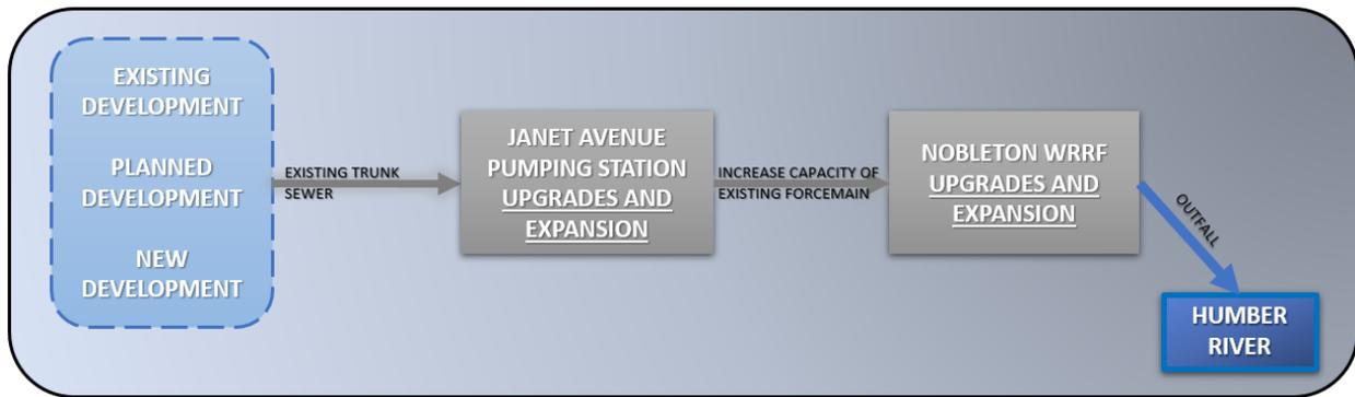
Figure 4-1: Alternative A: Expand and Upgrade the Existing Janet Avenue Pumping Station, Forcemain and Nobleton WRRF and Outfall
