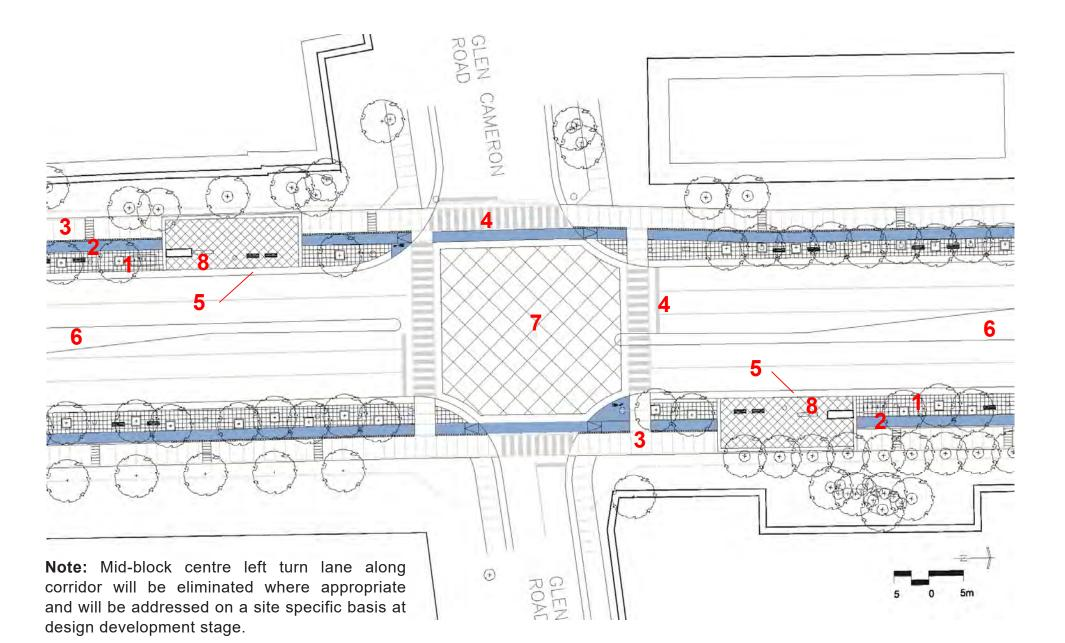
**Figure 54:** Detail Plan-Typical intersection w/In-boulevard Cycle Facility
