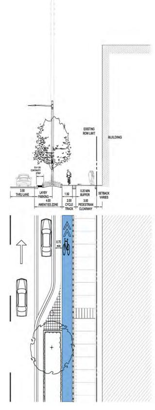
Figure 55: Option 1: Cycle Track protected by 2.5m lay-by parking with min. 0.7m "dooring zone" from cycling facilities and by min 0.2m buffer strip adjacent to Pedestrian Clearway.
