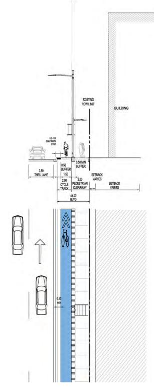
Figure 57: Option 3: Cycle Track protected by 0.5m min buffer strip within Continuity Strip adjacent to the roadway and by min 0.5m buffer strip adjacent to Pedestrian Clearway
