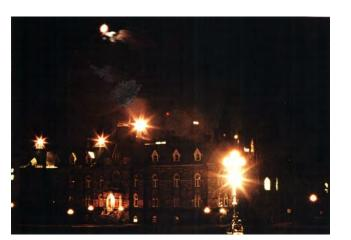
**Figure 119:** West Block, Parliament Hill: Glare vs. Visibility - Roof mounted security lights caused glare, obscuring view of the building and impairing security
