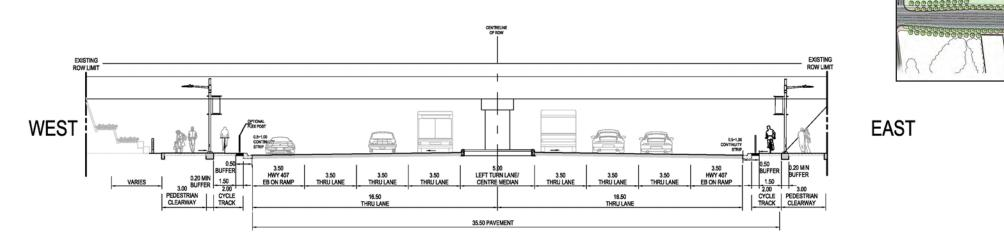
Figure 101: Concept C | Section I-I 407 w/Reduced Shoulder
