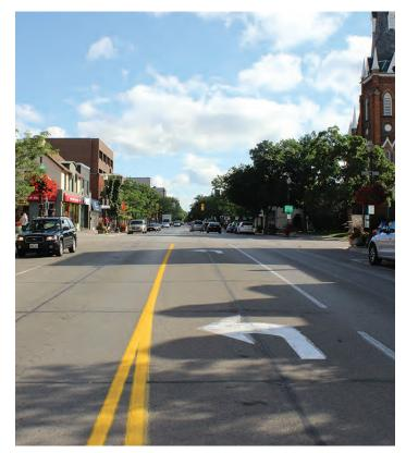
Left-turn lanes can reduce delays at intersections
