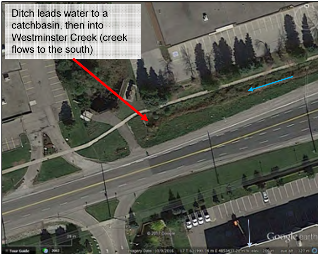
Zoomed Map #12 (Aerial): Langstaff Road West of Dufferin Street. Steady flow of water in ditch, 3-5 L/s observed on Sept. 21, 2017, during warm, dry weather. Source: Google Earth.
