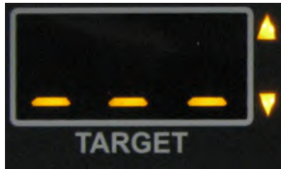
Figure 4.3.1e Both up and down Arrows display in Stationary All Mode when front or rear antenna is selected.
