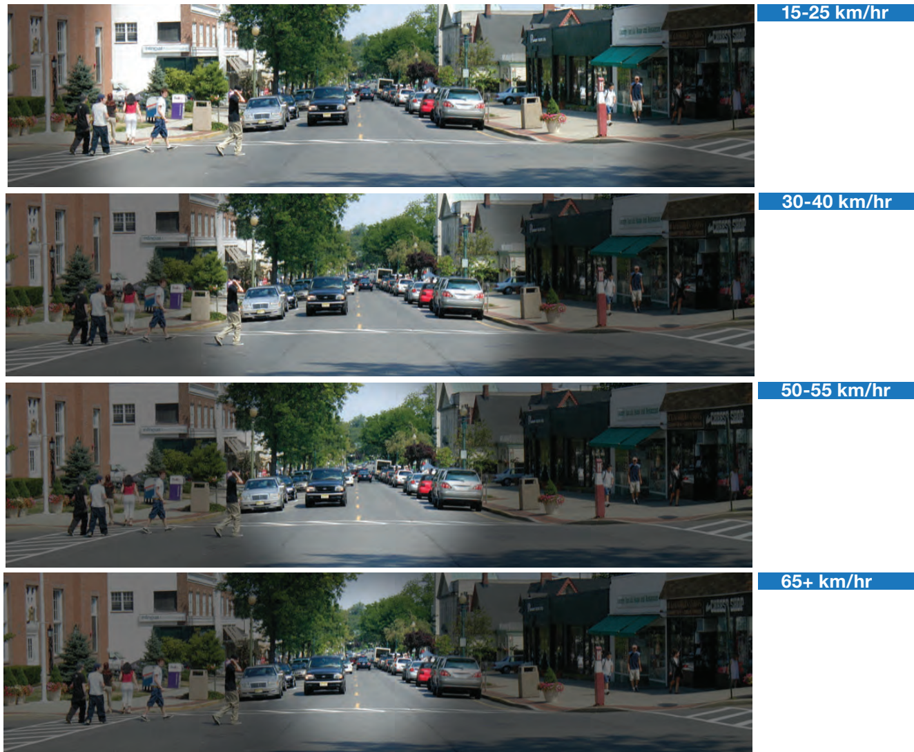
Figure 17. These images show the narrowing field of vision for drivers as vehicular speeds increase
