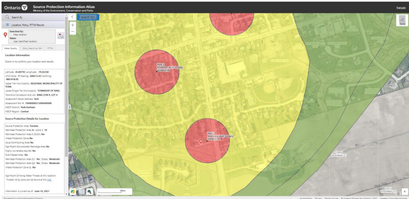
Figure 2 Source Protection Information Atlas (SPIA) map showing the location of the project activity with the highest vulnerability score (red pin). Vulnerability scores for groundwater protection zones are 10 (red), 6 (yellow) and 2 (green).
