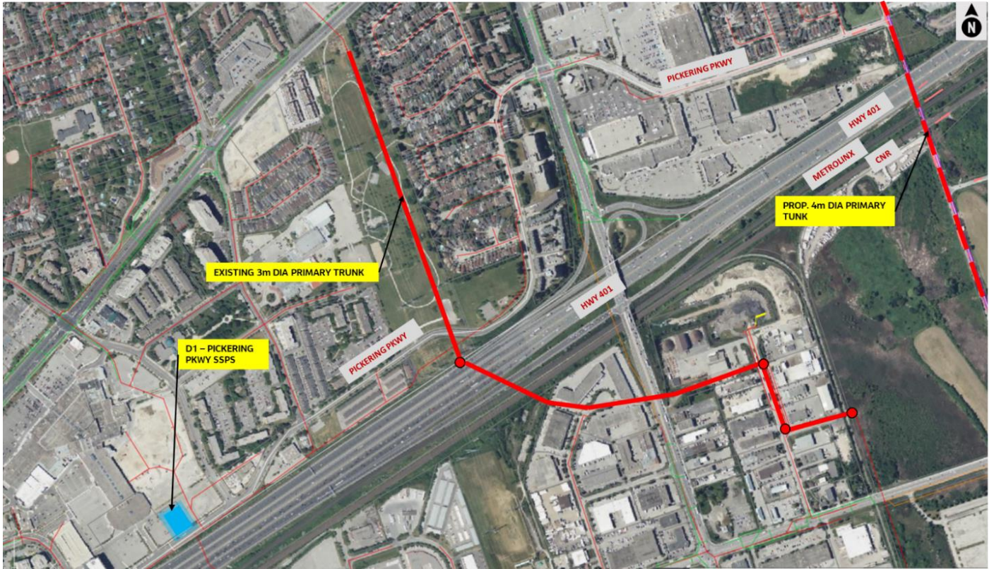
Figure 8.11 Pickering Parkway SPS Conceptual Schematic
