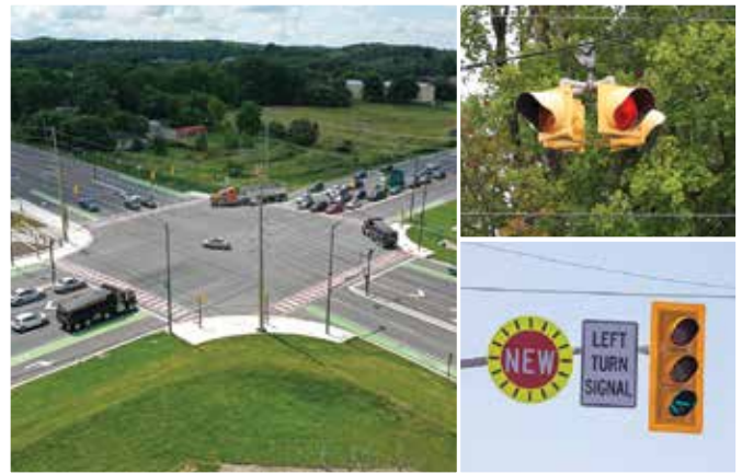
PHOTOS: LEFT – An intersection that shows clear sightlines. TOP RIGHT – Flashing beacons at an intersection. BOTTOM RIGHT – Left turn signal
