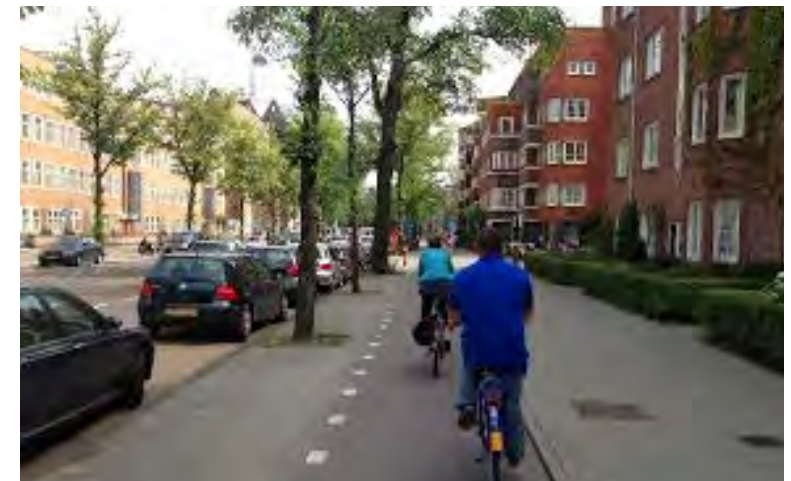
Figure 47: Lay-by Parking is located in-line with the Furnishing and Planting Zone
