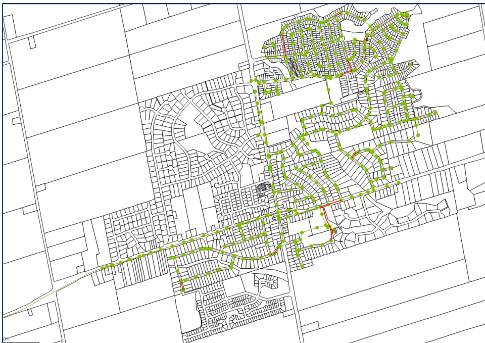
Figure 14 – Pipes which are surcharged during the design event for the existing system
