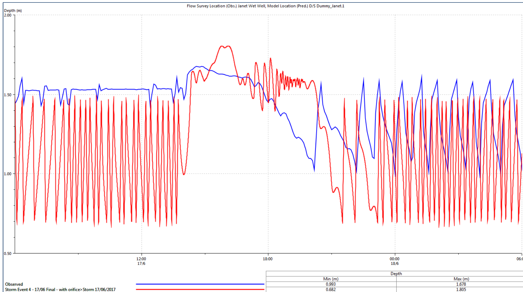
Figure A45: Storm event graph showing the comparison of the depth in Janet Avenue PS on 17/06/2017
