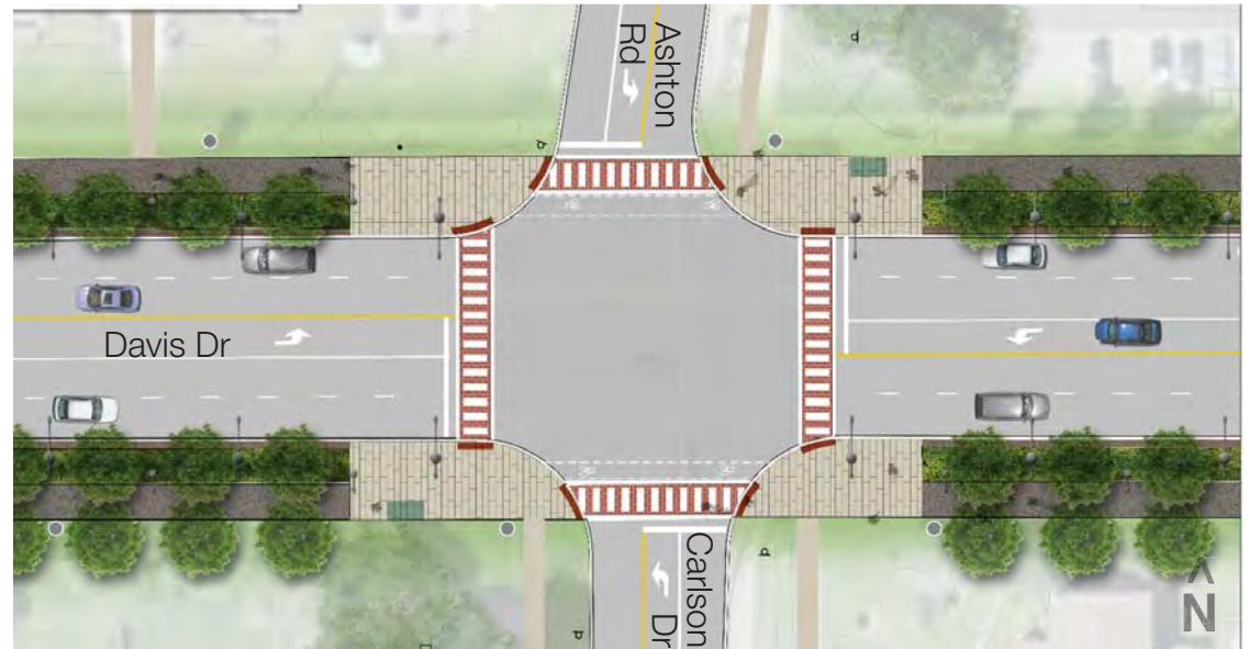
Plan of a signalized intersection along the Green segment of Davis Drive East
