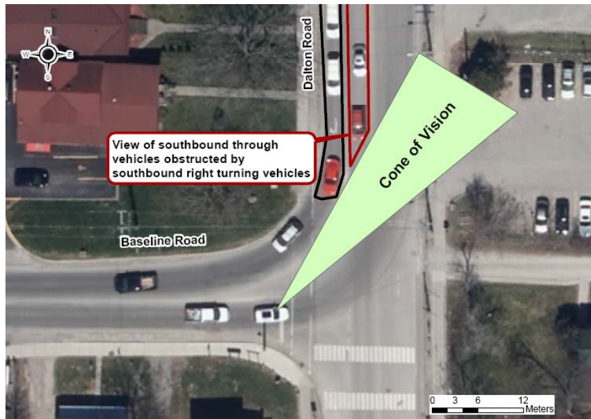
Figure 2 Illustration of Sight Line Obstruction
