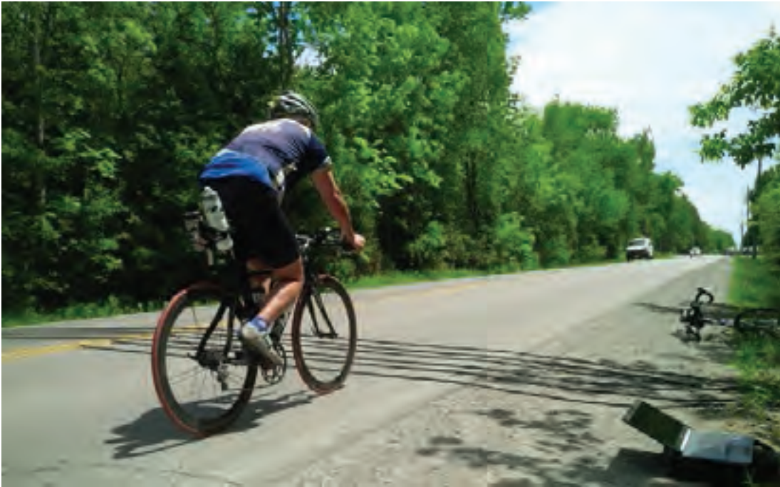
Example of Temporary Automatic Traffic Recorder tubes for bicycles
