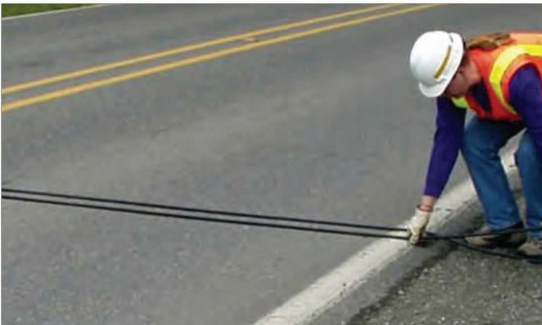
Example of Temporary Automatic Traffic Recorder tubes for cars, trucks and buses
