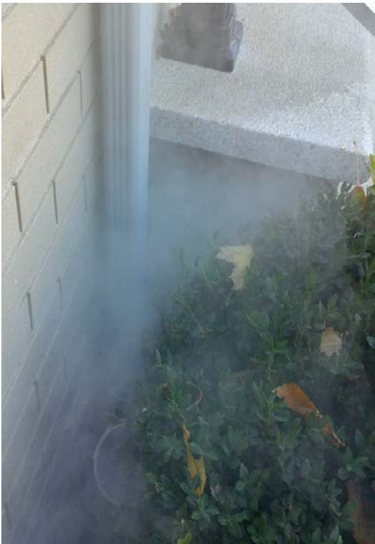
Figure 12 - Smoking Downspout and Open Sanitary Cleanout in Richmond Hill and Vaughan
